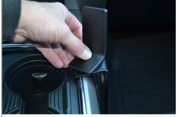
2. Hook the top left edge of the ProClip over the top right edge of the center console. See photo.
