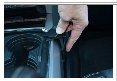
3. Press down on the right side of the ProClip and hook the lower right edge of the ProClip into the seam next to the gap opener.
